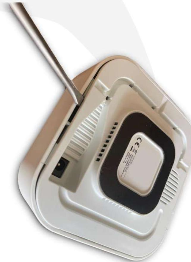
Please locate the SD card as shown in the image below. Remove the card and insert it into an SD card reader/adapter on your PC.
